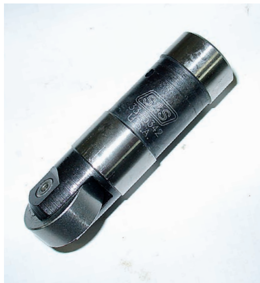
S&S hydraulic tappets feature a revised metering device which ensures rapid lifter pump-up.
