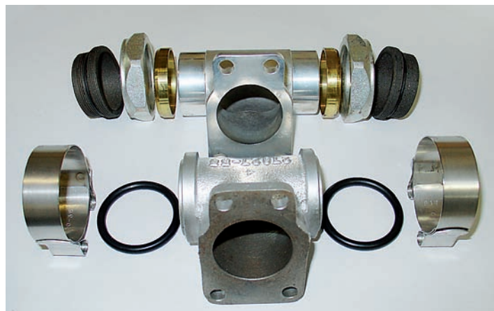
The early style of inlet manifold was replaced by this O-ring version in 1955.
